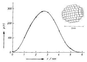
Fig. 2 Model structure and comparison of the experimental and model p(r)-functions of core CBH II. The functions are normalized to an integral of 105.
