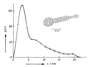
Fig. 1 Model structure and comparison of the experimental and model p(r)-functions of intact CBH II. The functions are normalized to an integral of  $10^{\circ}$ .
